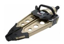
Constructed of high strength, aircraft grade, aluminum alloy forgings with a wear resistant anodized finish. The \$60-XL is evenly balanced at the cross bar and has a collapsible "D" handle. The shape of the tips incorporate three different angles to effectively grip throughout the arc of the spreading cycle. The tips are wider to reduce tearing during spreading. The \$60-XL has a variable speed, "deadman" control with load holding capability and over-pressurization relief.
