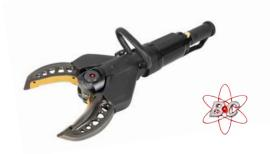
Constructed of ultra lightweight high strength, aircraft grade, aluminum alloy forgings. The blades on the C-195 NXTgen Cutter are forged steel with removable high strength inserts. The C-195 Cutter has a "D" handle that can be rotated 360 degrees or removed when working in confined spaces. The C-195 Cutter has a variable speed, "deadman" control with load holding capability and overpressurization relief.
