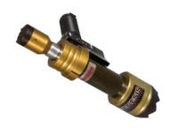
Constructed of high strength, aircraft grade, aluminum alloy with a wear resistant anodized finish. The 21 inch Push-Pull Ram has a variable speed, "deadman" control with load holding capability and over-pressurization relief. The 21 inch Push-Pull is also fully compatible with the Slip-Fit Ram Accessory kit.
