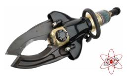
Constructed of high strength, aircraft grade, aluminum alloy forgings with a wear resistant anodized finish. The blades on the ALL-9 Cutter are forged steel. The ALL-9 Cutter has a "D" handle that can be rotated 360 degrees or removed when working in confined spaces. The ALL-9 Cutter has a variable speed, "deadman" control with load holding capability and over-pressurization relief. The ALL-9 is the only tool capable of rating all 9's in NFPA 1936 standard.
