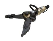
Constructed of high strength, aircraft grade, aluminum alloy forgings with a wear resistant anodized finish. The 17C BRUTE is evenly balanced at the cross bar and has a collapsible "D" handle. The shape of the tips incorporate three different angles to effectively grip throughout the arc of the spreading cycle. The tips are wider to reduce tearing during spreading. The 17C has a variable speed, "deadman" control with load holding capability and overpressurization relief.
