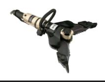
Constructed of high strength, aircraft grade, aluminum alloy forgings with a wear resistant anodized finish. The 15C is evenly balanced at the cross bar and has a collapsible "D" handle. The shape of the tips incorporate three different angles to effectively grip throughout the arc of the spreading cycle and are also removable. The tips are wider to reduce tearing during spreading. The 15C has a variable speed, "deadman" control with load holding capability and over-pressurization relief.
