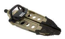
Constructed of high strength, aircraft grade, aluminum alloy forgings with a wear resistant anodized finish. The S49-XL is evenly balanced at the cross bar and has a collapsible "D" handle. The shape of the tips incorporate three different angles to effectively grip throughout the arc of the spreading cycle. The tips are wider to reduce tearing during spreading. The S49-XL has a variable speed, "deadman" control with load holding capability and over-pressurization relief.
