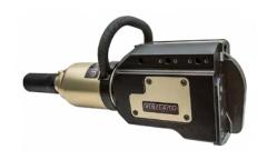
Constructed of high strength, aircraft grade, aluminum alloy forgings with a wear resistant anodized finish. The blade on the MT Cutter are forged steel. The MT Cutter has a "D" handle that can be rotated 360 degrees or removed when working in confined spaces. The MT Cutter has a variable speed, "deadman" control with load holding capability and over-pressurization relief. The MT cutter is ideal for incendents that involve mass transit vehicles such as buses,trains, and semi trucks
