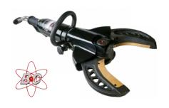
Constructed of ultra lightweight high strength, aircraft grade, aluminum alloy forgings. The blades on the c-236 Cutter are forged steel with removable high strength inserts. The C-236 Cutter has a "D" handle that can be rotated 360 degrees or removed when working in confined spaces. The C-236 Cutter has a variable speed, "deadman" control with load holding capability and over-pressurization relief.
