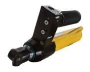
Constructed of high strength, aircraft **SPECIFICATIONS** grade, aluminum alloy forgings with a wear resistant anodized finish. The 15-30 Telescopic Ram has a variable speed, "deadman" control with load holding capability and over-pressurization relief.
