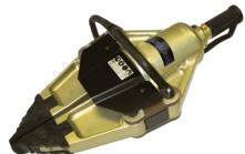
Constructed of high strength, aircraft grade, aluminum alloy forgings with a wear resistant anodized finish. The S80-XL is evenly balanced at the cross bar and has a collapsible "D" handle. The shape of the tips incorporate three different angles to effectively grip throughout the arc of the spreading cycle. The tips are wider to reduce tearing during spreading. The \$80-XL has a variable speed, "deadman" control with load holding capability and over-pressurization relief.
