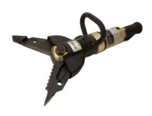
Constructed of high strength, aircraft grade, aluminum alloy forgings with a wear resistant anodized finish. The 14C is evenly balanced and has a rotating 360 degree "D" handle. The tips are wider to reduce tearing during spreading. The 14C has a variable speed, "deadman" control with load holding capability and over-pressurization relief.
