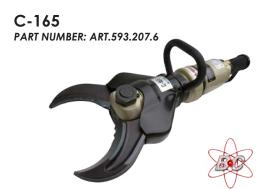
Constructed of high strength, aircraft grade, aluminum alloy forgings with a wear resistant anodized finish. The blades on the C-165 Cutter are forged steel. The C-165 Cutter has a "D" handle that can be rotated 360 degrees or removed when working in confined spaces. The C-165 Cutter has a variable speed, "deadman" control with load holding capability and over-pressurization relief.
