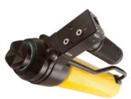
Constructed of high strength, aircraft grade, aluminum alloy forgings with a wear resistant anodized finish. The 19-51 3-Stage Telescopic Ram has a WIDTH(IN/MM) - 8.7/221 variable speed, "deadman" control with load holding capability and over-pressurization relief.
