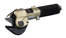
Constructed of high strength, aircraft grade, aluminum alloy forgings with a wear resistant anodized finish. The blades on the C-30 Mini Cutter are forged steel. The C-30 Mini Cutter has a variable speed, "deadman" control with load holding capability and overpressurization relief. The C-30 Mini Cutter is our smallest cutter and is a must have for cutting in tight spaces inside vehicles.
