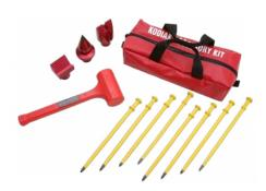
The Kodiak Accessory kit features 3 new heads designed to make stabilization easier. The Conical Point head can be driven into sheet metal with the deadblow hammer. This allows the Kodiak to be placed on fenders, doors, roofs or anywhere a heavy sheet metal "skin" can be punctured. The Chain Wedge head allows the Kodiaks to be used with the HD #2 chain kit or any 3/8" chain and hook assembly. The V-head allows the Kodiaks to be placed more securely along rails and frames of overturned vehicles.
