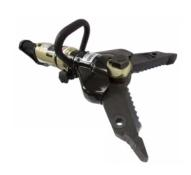
Constructed of high strength, aircraft grade, aluminum alloy forgings with a wear resistant anodized finish. The 14C is evenly balanced and has a rotating 360 degree "D" handle. The tips are wider to reduce tearing during spreading. The 14C has a variable speed, "deadman" control with load holding capability and over-pressurization relief.
