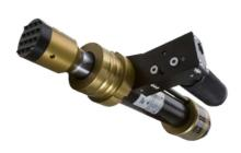
Constructed of high strength, aircraft grade, aluminum alloy with a wear resistant anodized finish. The 31 inch Push-Pull Ram has a variable speed, "deadman" control with load holding capability and over-pressurization relief. The 31 inch Push-Pull is also fully compatible with the Slip-Fit Ram Accessory kit.
